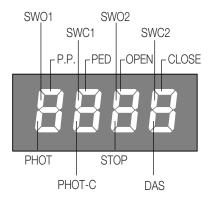
N.C. inputs are represented by the vertical segments. N.O. inputs are represented by the horizontal segments.
